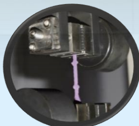
Pneumatic grips for Tensile test on rubber-base materials
